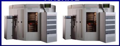
STK PowderHorns (2), managed by Cray DMF 2.8 PB max capacity
