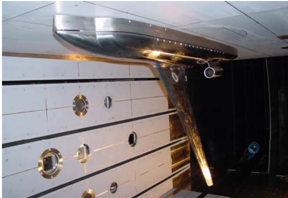
Cryotechnic test of generic Falcon shape in ETW
