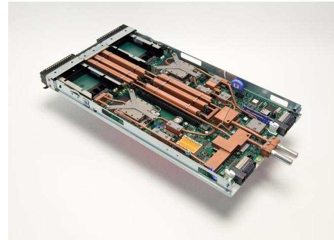
LRZ SuperMUC compute unit (cooling pipeline)
