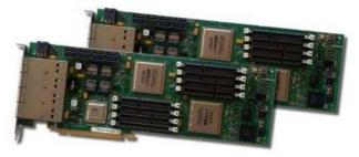
For less than a kW, the TERABOX provides up to 20 TeraFLOPS of total processing power, along with 6.5 Terabits/sec of memory bandwidth and 1.28 Terabits/sec of I/O (up to  $128 \times 10$ GigE or  $32 \times 40$ GigE links) all in a very compact 5U rackmount solution. This low power, highly flexible system, fully tested and configured, is ideal for demanding power processing and high density network applications and comes instantly ready for HPC application development.
