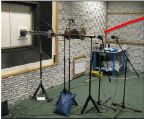
Tailpipe measurement test bench.
