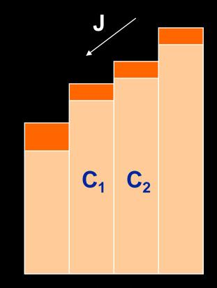
dx In each volume element, an equilibrium calculation is performed. These calculations are independent and can be parallelized
