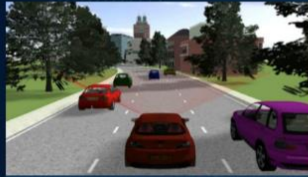
Pedestrian AEB based on radar-camera fusion
