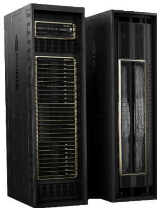
Nvidia GB200 NVL72 cluster 1.4 FP4 EFLOPs, 150 kW
