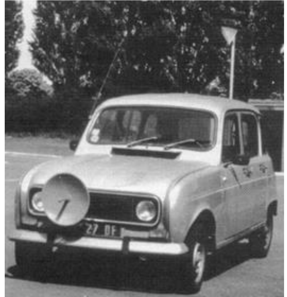
Test Vehicle Renault 4L with anti collision prototype radar
